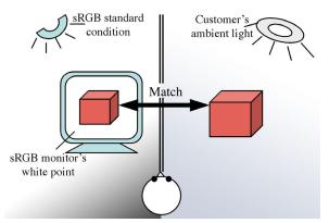
Figure 2. Haploscopic matching method used in the previous experiment for the spectral turn technique applied with the single chromatic adaptation model in RLAB model.
