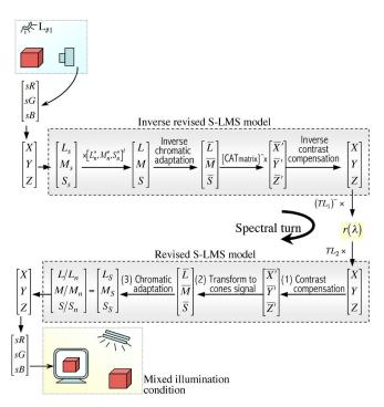
Figure 4. The spectral turn method applied with the mixed chromatic adaptation model: revised S-LMS model.
