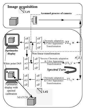
Figure 1. The process of spectral based processing for sRGB system.
