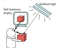
Figure 3. Human visual system adapted partially under the mixed illumination condition (as in the simultaneous binocular matching method).
